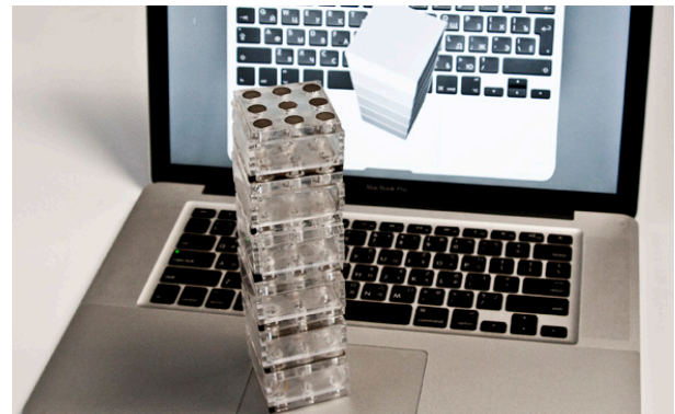
Figure 10: Switching to a less sensitive capacitive sensor allows us to stack 6 CapStones (touch pad of a MacBook Pro).
