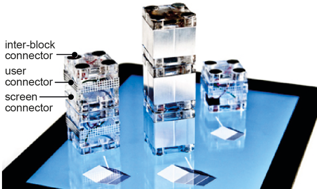
Figure 3: Each CapStone features three types of connectors (here a design featuring 2x2 screen connectors).
